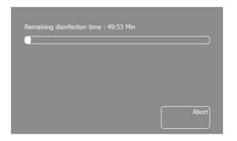
• Press the "Abort" button on the Disinfection Remaining Time screen.
