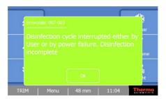
Press the "OK" button to remove the error message.
