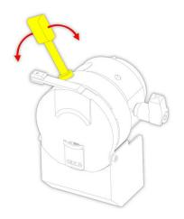
• Use the orientation handle to orient the specimen on the x- and y-axes.
