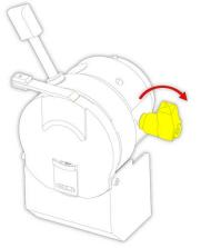
• Tighten the specimen head clamping lever again.
