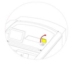
• Open the Cold D reservoir cover to access the filling inlet of the disinfectant tank.
