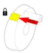
• The mechanical hand brake lock acts as a safety device, especially when the instrument is turned off. The mechanical hand brake lock can be activated by a slider on the handwheel.
