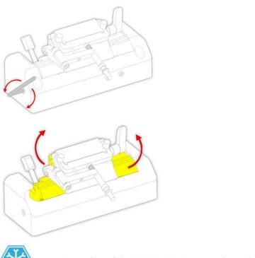
Loosen the clearance angle adjustment screw on the lower left side of the blade holder using the Allen key 5mm provided
