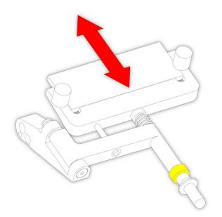
• To raise the height of the Anti Roll Plate, turn the screw anti clockwise.
