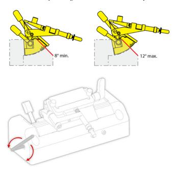
• Re-tighten the clearance angle adjusting screw to fix the selected clearance angle.
