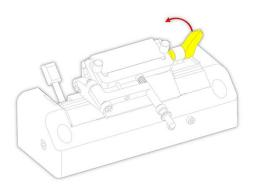
• Push the blade clamping lever towards the back of the instrument to clamp the blade in position.
